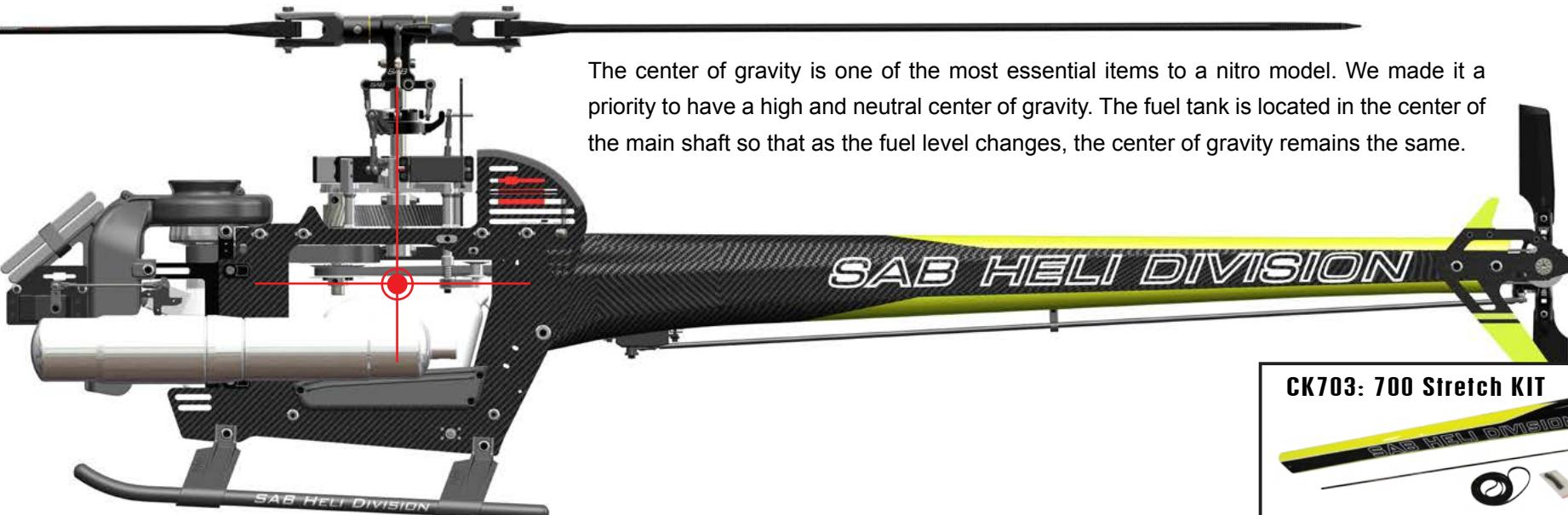
The center of gravity is one of the most essential items to a nitro model. We made it a priority to have a high and neutral center of gravity. The fuel tank is located in the center of the main shaft so that as the fuel level changes, the center of gravity remains the same.
